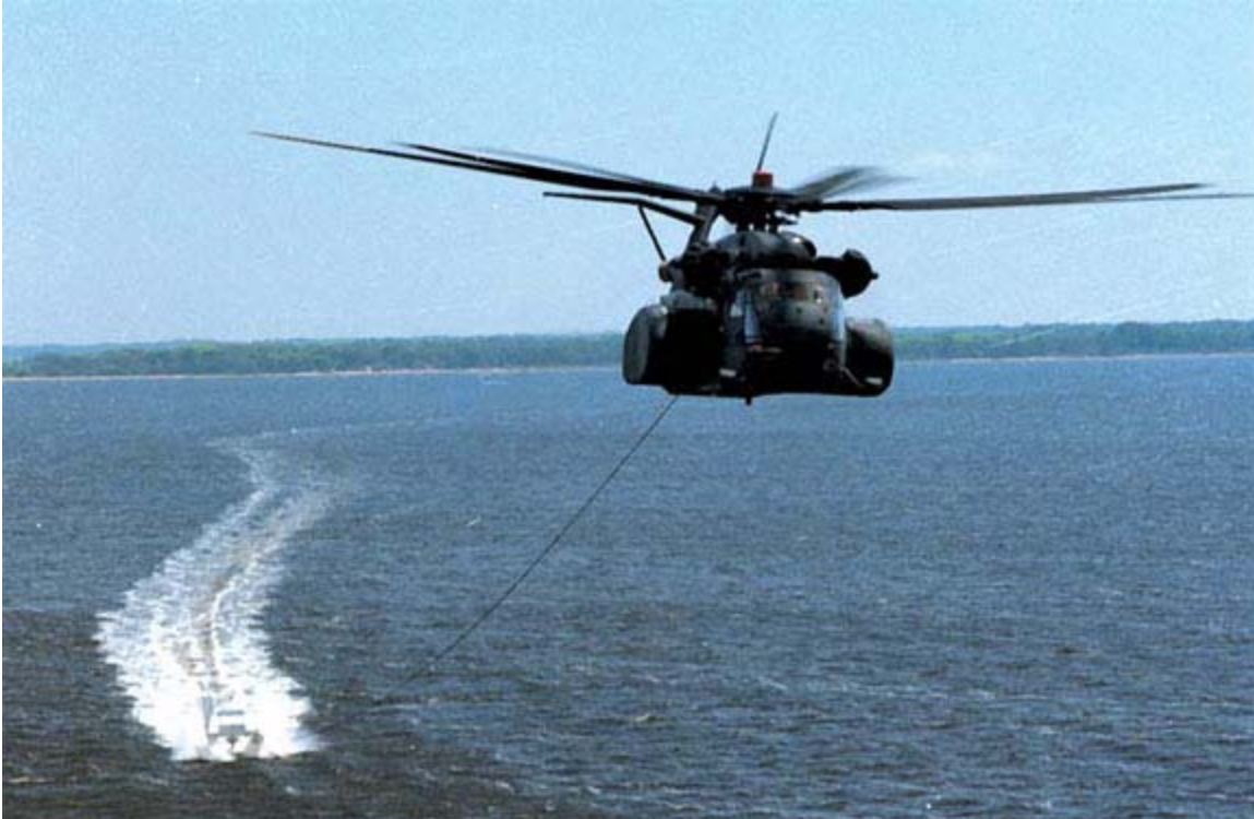
Minesweeping is a method of active maritime countermeasure and is conducted by either surface craft or helicopter.
